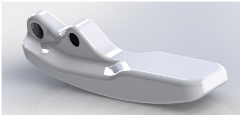
Figure 6. Version 3.11 of the foot. There is increased space in the front of the foot for the PCB. There is an increased thickness from the Achilles hole to the top of the foot. There are larger fillets in the front and back corners of the foot.
