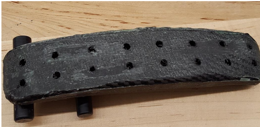
Figure 25. The holes on the foot after being drilled out using the jig.
