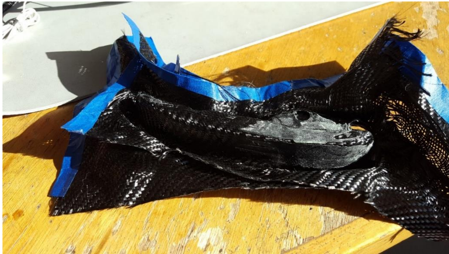
Figure 23a. An insufficient amount of epoxy was used to create the foot. Some parts of the foot still has the texture of the woven carbon fiber.
