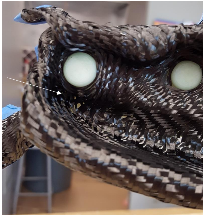
Figure 12. The carbon fiber wrapped around the ankle and Achilles hole extrusion. The carbon fiber in the bottom corner of the foot is sparse, marked by the arrow. This issue was a common issue in both the front and back of the mold made from foot v3.8.
