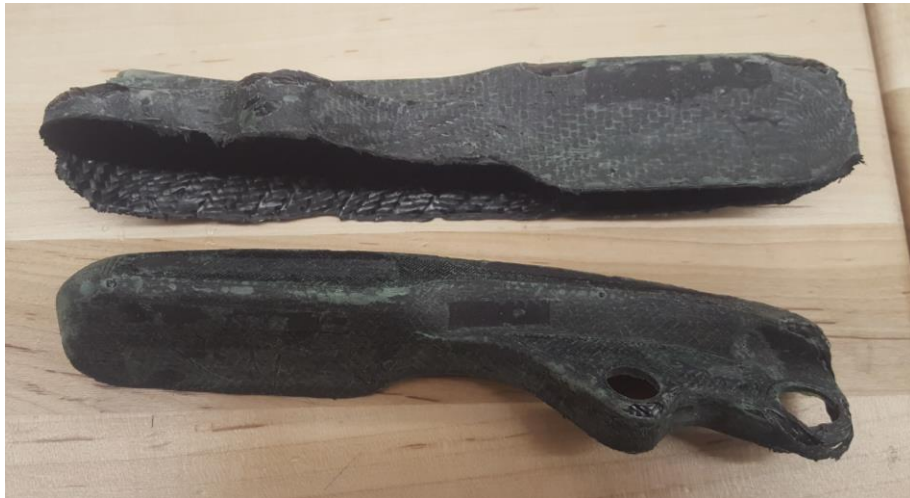
Figure 24. Both halves of the feet after being trimmed of excess carbon fiber.
