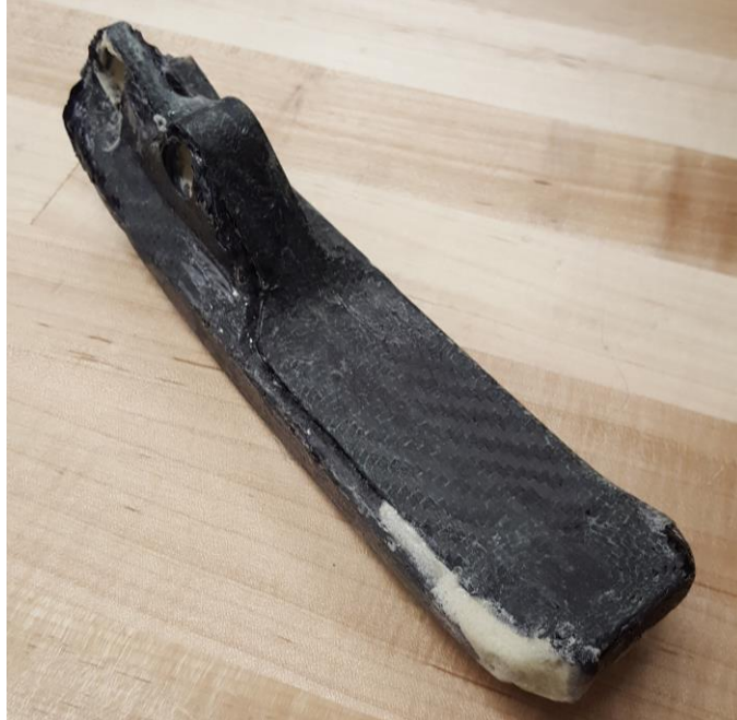
Figure 27. The foot after foam has been poured in. The foam can be seen on the exterior of the foot because the two pieces of the foot were not vacuum sealed properly before the pouring of the foam.
