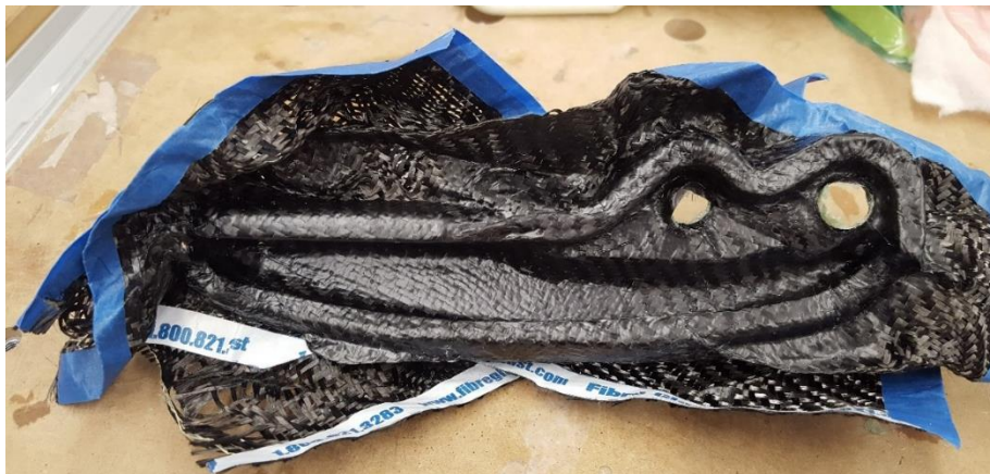
Figure 23b. A sufficient amount of epoxy applied.
