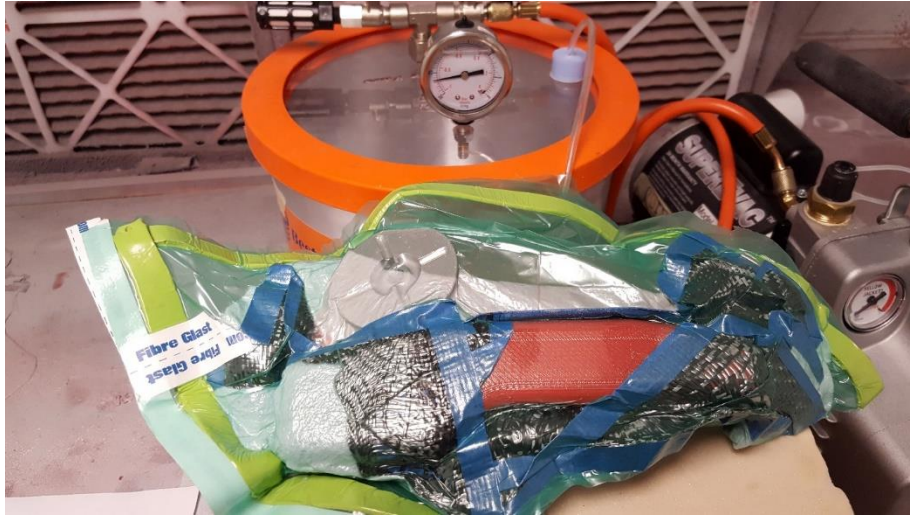
Figure 19. The mold is inverted once the pressure in the vacuum bag is sufficient in order to make sure the epoxy is distributed through the entire foot and is not just pooled on the side of the foot.
