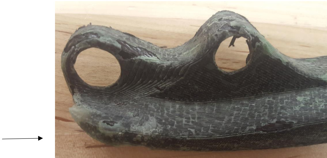
Figure 13. A region of no carbon fiber can be seen, marked by the arrow.
