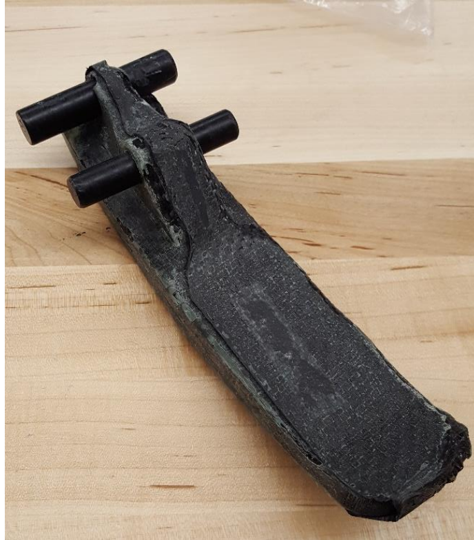
Figure 26a. Assembled foot. The Delrin rods are used to make sure that the holes are the right size.
