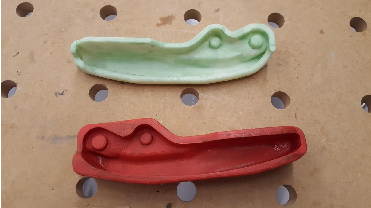
Figure 10. The molds after the mold release is applied. The mold release turns the initially white mold into a greenish color. This color change is less apparent if the mold is not white to begin with.
