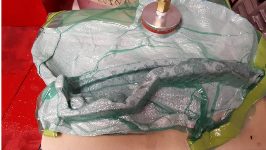
Figure 21. Black spots of excess epoxy pockets can be seen on the mold.
