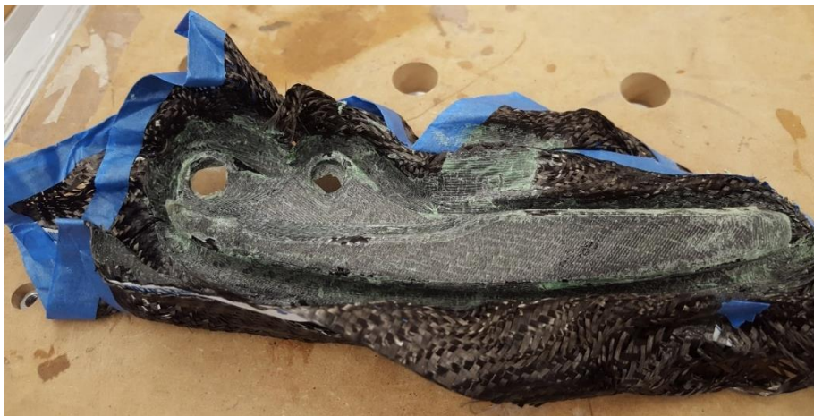
Figure 23b. A sufficient amount of epoxy applied.
