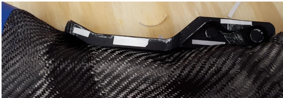
Figure 15. Double sided tape was applied on the mold before the first layer of the carbon fiber is placed into the mold.
