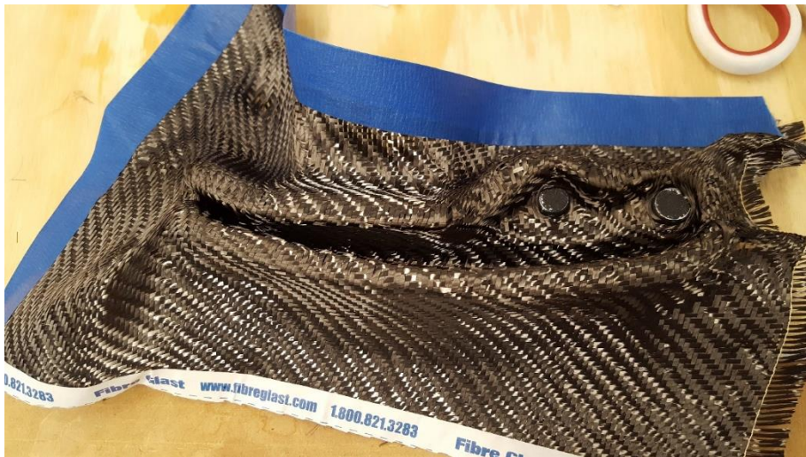
Figure 17. The first layer of the carbon fiber is placed into the mold.
