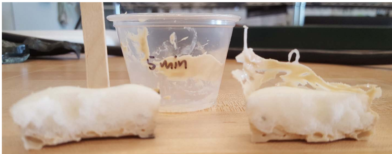
Figure 21a. The brush on polyurethane and the Flex Foam-it! 17 foam combined 5 minutes after the brush on polyurethane had sat for 5 minutes.
