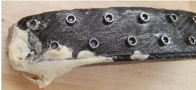
Figure 18. The foot after foam has been poured in. The foam can be seen on the exterior of the foot because the two pieces of the foot were not vacuum sealed properly before the pouring of the foam.
