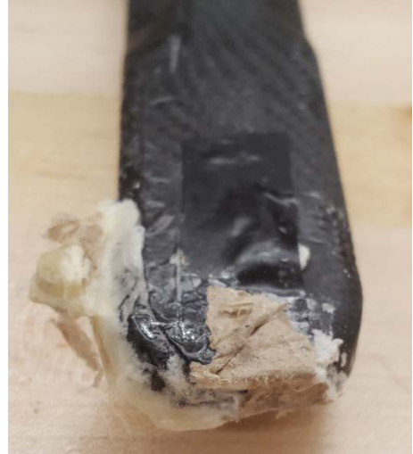
Figure 18. The foot after foam has been poured in. The foam can be seen on the exterior of the foot because the two pieces of the foot were not vacuum sealed properly before the pouring of the foam.
