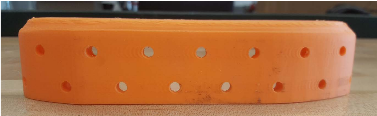
Figure 12b. Actual jig to create the holes for the pressure sensors in the outer mold, bottom view.
