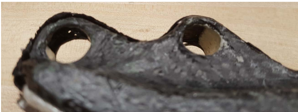
Figure 20. The ankle and achilles hole region after the 6lb foam has been poured.
