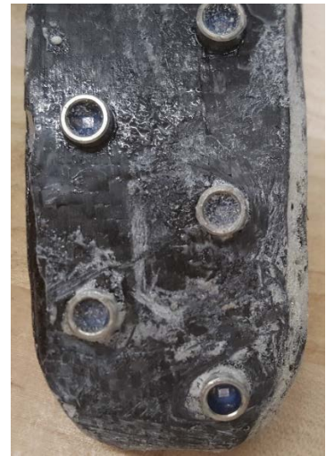
Figure 19. The foot after the excess foam has been removed.
