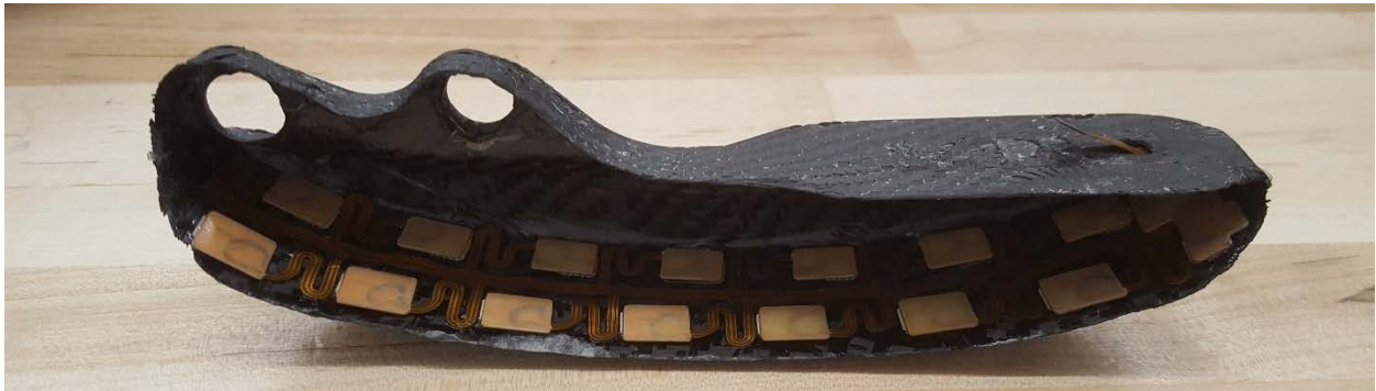
Figure 16a. The flexible PCB epoxied onto the foot.
