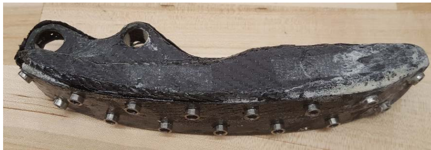
Figure 19. The foot after the excess foam has been removed.
