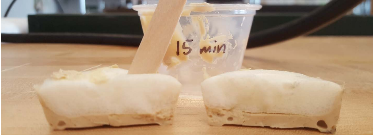
Figure 21b. The brush on polyurethane and the Flex Foam-it! 17 foam combined 5 minutes after the brush on polyurethane had sat for 15 minutes.
