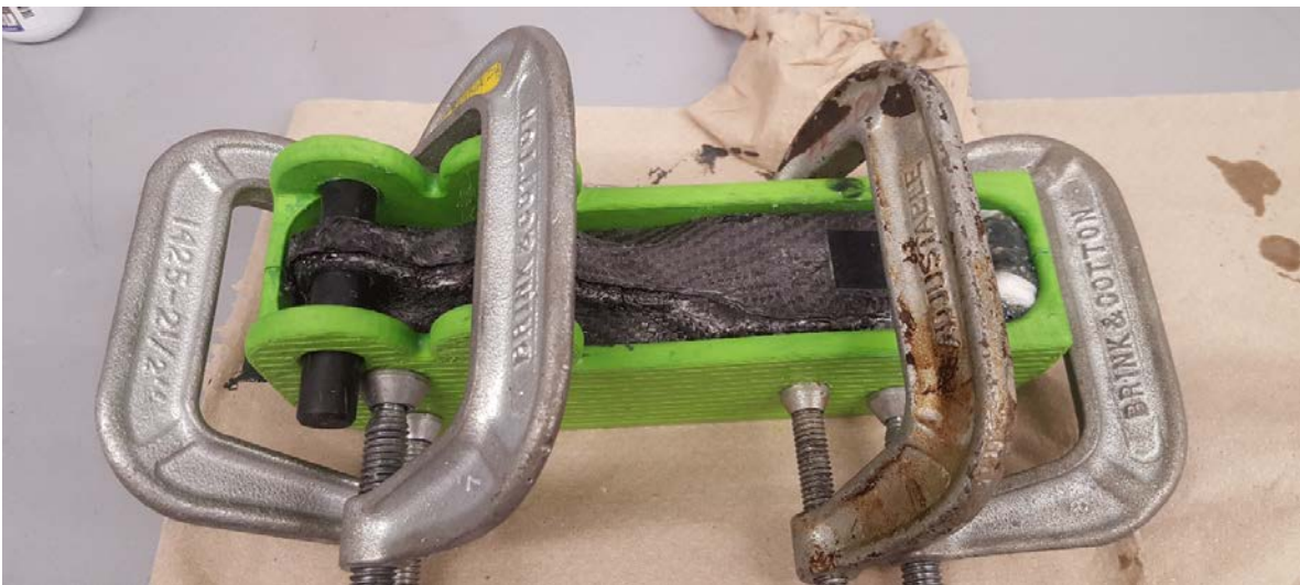
Figure 22. The setup to create the foam shoe. Clamps are used to hold the two pieces of the mold in place.
