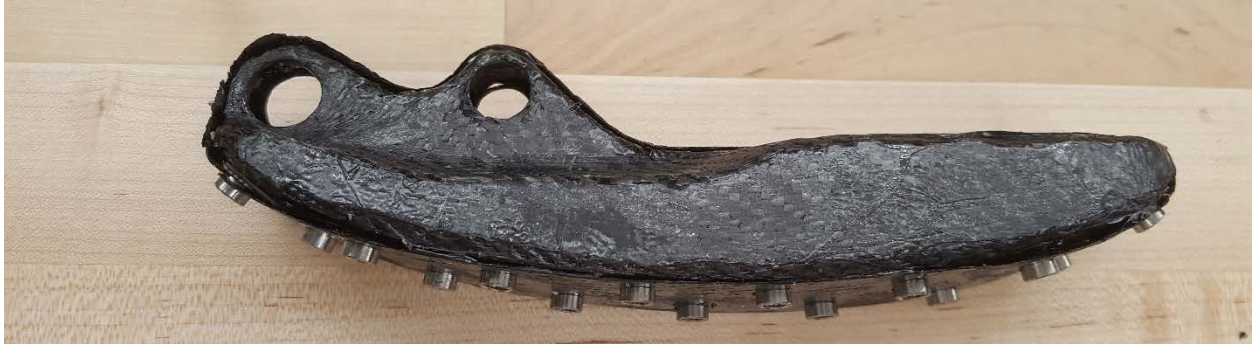
Figure 17b. The foot after the two halves have been epoxied together, profile view.
