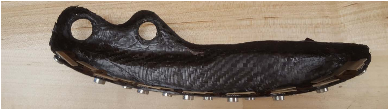
Figure 16b. The flexible PCB epoxied onto the foot, side view.
