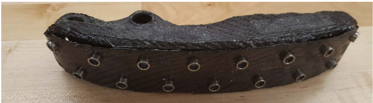
Figure 17a. The foot after the two halves have been epoxied together.
