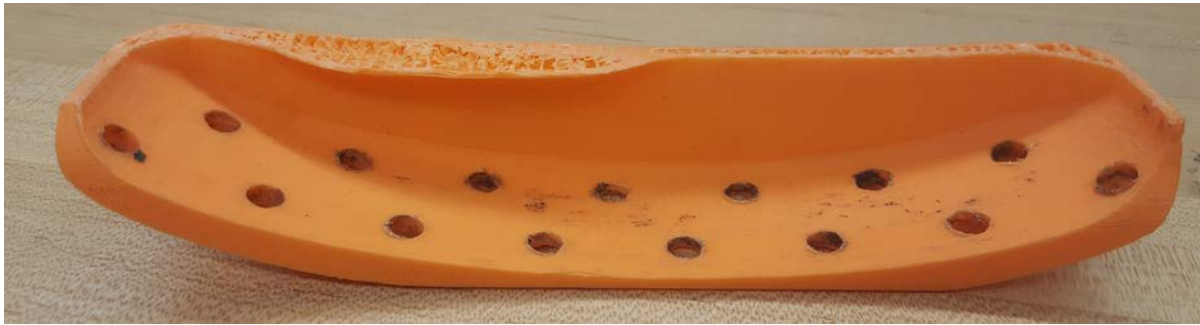
Figure 12a. Actual jig to create the holes for the pressure sensors in the outer mold.
